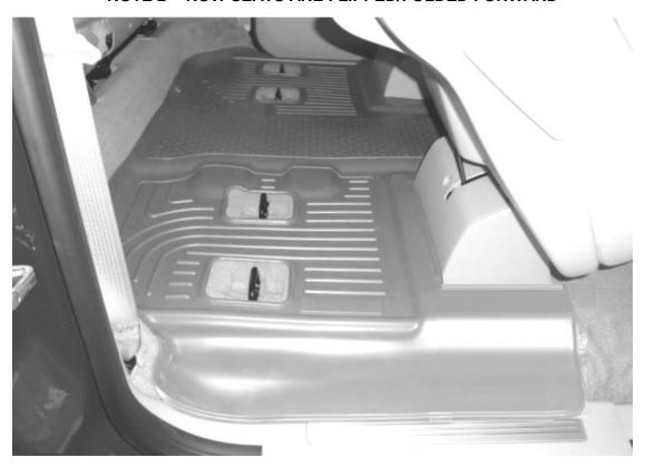
NOTE SEAT ATTACHES TO FLOOR THROUGH LINER
