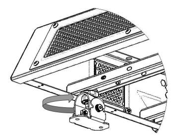
• Do not fully tighten 3/8" Hex head bolt.
