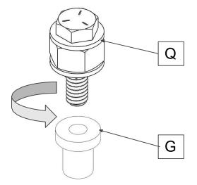
• Hand tighten ¼" rivet nut onto installation tool as shown.
