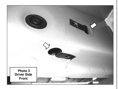
**Step-3** Attach one of the brackets to the rocker panel using (2) M8 hex bolts, (Photo 4 & 5). Leave the bolts loose for final adjustment.
