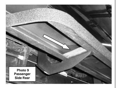
**Step-7** Align the running board with the vehicle and tighten all supplied nuts and bolts securing the running board and bracket assembly. Repeat the installation steps to install the driver side brackets and running board. Remember to check and retighten all bolts periodically.
