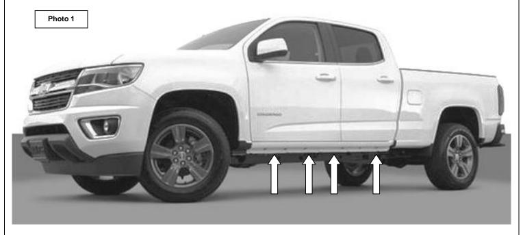
**Step-1** Begin the installation on the driver side. Starting at the front of the vehicle, locate and remove the plastic plugs in the back side and bottom of rocker panel to expose the holes used for placement of the M8 Clip- Nuts, (Photo 2).
