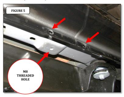
**Step-4** Attach one of the driver side Front/Center brackets to the pinch mold using (2) 1/4" x 1" hex head bolts, (4) 1/4" flat washers, (2) 1/4" lock washers and (2) 1/4" hex nuts, and to the underside of the body using (1) M8 x 25mm hex bolt, (1) 5/16" lock washer and (1) 5/16" flat washer, (FIGURE 6 & 7). Leaves the nuts and halts leave for final adjustment.
