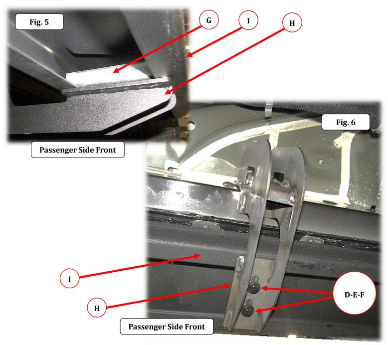
**Step-5** Align the running board with the vehicle and tighten all supplied nuts and bolts securing the running board and bracket assembly. Repeat to install the brackets and running board on the driver side of the vehicle.
