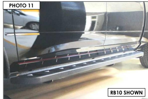
11. Align the running board with the vehicle and tighten all supplied nuts and bolts securing the running board and bracket assembly, **(Photo 11)**. Repeat the installation steps to install the passenger side brackets and running board. Remember to check and retighten all bolts periodically.
