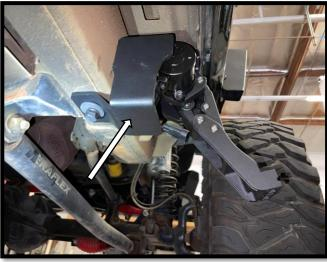
**Step 10**: Install the passenger side front motor protective bracket. Secure the protective bracket using an M12 hex bolt, flat washer, and lock washer. Torque to 25 ft-lbs.
