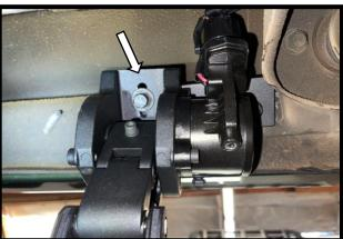
**Step 6**: Install rear passenger side bracket onto weld seam using (2) M8x20MM Hex Bolts, M8 Lock Washer, M8 Flat Washer. On the underside of the bracket, secure it to the motor to the mounting plate using (1) M8x35MM Hex Bolts, M8 Lock Washer, M8 Flat Washer.
