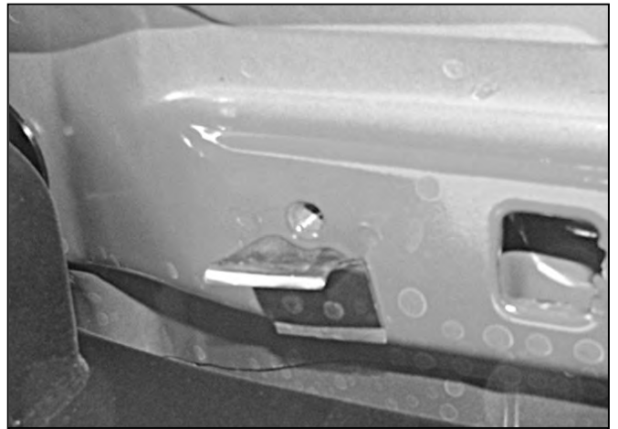
(Fig 2) M8 threaded hole in floor frame channel (passenger side-front pictured for example)
