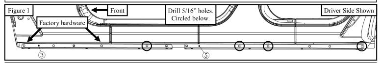
3. Secure the both pinch weld adapters onto the vehicle pinch weld using the factory hardware present and the provided M6 hardware (Items 15-18). Align and adjust as necessary and then tighten M6 hardware to 5-7 ft-lbs. See **Figures 2 - 3.**
