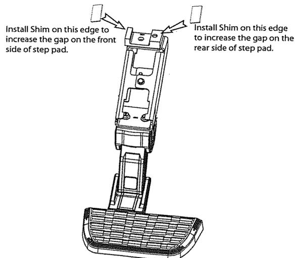
Install Shim on this edge to increase the gap on the front side of step pad.
