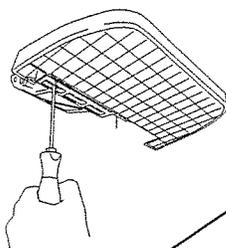
Adjust step pad to be in line with fender.
