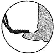
To retract, gently kick up on the underside of the step pad.
