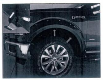
STEP 8: Place the Fender Flare onto the vehicle and fit into the correct position following the contours of the body. Use 2 of the retaining clips and 5.5mm bolts to secure the Fender Flare to the body. Make sure the clip securely engages the Fender Flare.
