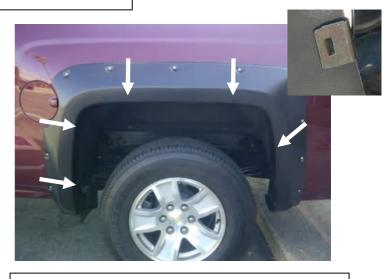
**STEP 9:** To secure the Fender Flare to the body, apply upward tension on Fender Flare to the vehicle fender when installing the black metal clips. Slide the clips over the Fender Flare and the inner wheel arch lip in the five locations shown. Position the clip so that the barb in the clip locates in the slot of the Fender Flare.
