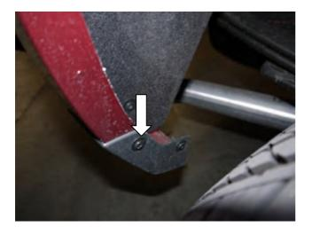
**STEP 8:** Using #15 Torx head screwdriver remove upper screw from the rear factory mudguard. Maintain screws for re-install.
