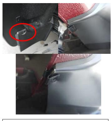
**STEP 16:** Install the "E" shape clip so that the clip slides over the inner sheet metal lip and is in line with the slot in the underside of Fender Flare. To secure the clip to Fender Flare apply inward tension on Fender Flare to the vehicle fender, position the clip so that the barb in the clip locates in the slot of the Fender Flare. Tighten previously loosened #15 torx screw in aero spoil.
