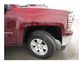
**STEP 1:** Clean the body areas where the Fender Flares will make contact. Ensure fenders are dry prior to install. Turn tires outward for Fender Flare installation.
