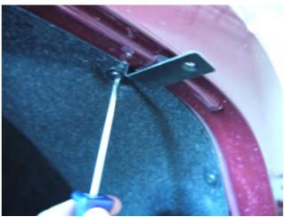
**STEP 4:** Apply clear tape to the inside edge of the fender wheel arch in front of positions **A**, **B** and **C** (step 5) over mastic sealant. Install the large brackets in positions **A**, **B** and **C** (step 5) aligning the slot in the bracket with the vacant holes from the factory screws in the vehicle wheel arch. Ensure clips are positioned over the clear tape. Re-install the factory screws in location **A**, **B** and **C** using a #15 Torx head screwdriver.
