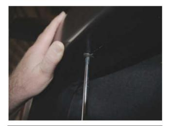
**STEP 5:** Place Fender Flare on the vehicle into the position of best fit so the slots in position **A** and **B** are over the holes in the front end of large clips. Ensure bottom rear slot in Fender Flare is located over the vacate hole in the factory mudguard. Apply upward tension on Fender Flare to the vehicle fender when Installing the screws and washers provided into the clips in position **A** and **B** using a Philips head screwdriver.
