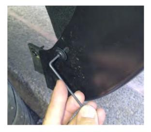
**STEP 17:** Using #15 Torx head screwdriver re-install the upper screw from the rear factory mudguard through the slot in the Fender Flare. Ensure all fixing points are tight and secure and that the rubber seal is flush neatly against the vehicle body.
