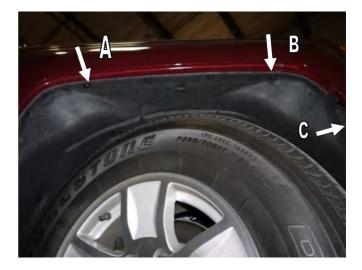
**STEP 2:** Place Fender Flare on the vehicle into the position of best fit. Note where the slots in Fender Flare at positions **A**, **B** and **C** align with the existing screws in the vehicle wheel arch. Remove Fender Flare. Remove the existing vehicle screws in location **A**, **B** and **C** using #15 Torx head screwdriver. Maintain screws for re-install.
