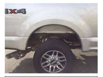
**STEP 5:** Clean the body areas where the Fender Flares will makes contact. A light misting on fender using a soap and water solution can aid in proper rubber placement.
