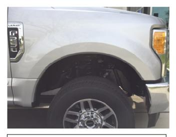
**STEP 1:** Clean the body areas where the Fender Flares will makes contact. A light misting on fender using a soap and water solution can aid in proper rubber placement.
