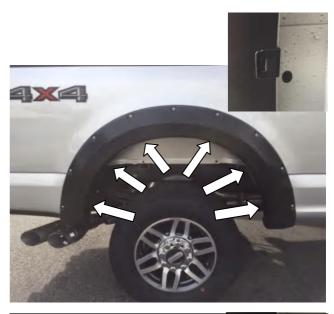
**STEP 6:** Place the Fender Flare onto the vehicle and fit into the correct position following the contours of the body. Use six (6) provided "U" Shaped Retention Clips to secure the Fender Flare to the body. Ensure the barb in the clip securely attaches in the slot on the Fender Flare. REPEAT ALL ABOVE STEPS FOR OPPOSITE SIDE OF VEHICLE.
