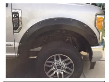
**STEP 3:** Place the Fender Flare onto the vehicle and fit into the correct position following the contours of the body. Ensure the slots in the part align with the holes in the fender from the previously removed 7/32" socket head screws.
