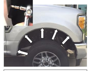
**STEP 2:** Remove all five (5) 7/32" socket head screws and retain for installation of Fender Flares.
