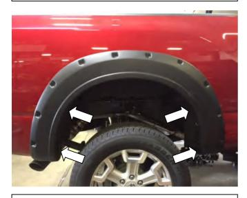
**STEP 10:** Place Fender Flare on the vehicle into the position of best fit. Note where (4) slots in Fender Flare correspond with (4) existing screws in the vehicle wheel arch. Remove Fender Flare. Remove only the existing vehicle screws in location as shown with a #2 Phillips head screwdriver. Maintain screws for re-install.
