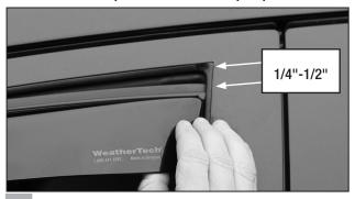
Insert the rear edge leaving a gap at the top.
