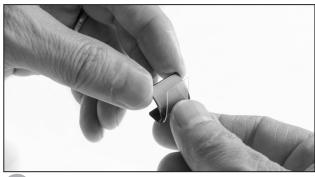
Place one strip of the provided clear tape centered onto the top of the weather strip clip.
