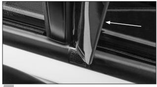
With the deflector now resting on the weather strip clip, slide forward into the channel. Ensure edge rests on top of the weatherstrip clip.
