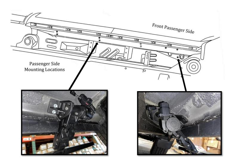
**Step 3**: Install the Rear passenger side motor using (2) M8X30mm Flange Bolts, to fasten the motor to the vehicle. Use the rear center mounting hole location. The hardware should be hand tightened only until snug. This will allow the motor assembly to move and align easier when installing the running board.
