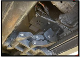
**Step 5**: Install the Rear Bracket and control module (sandwiched together) on passenger side using (2) M8X30mm Flange Bolts, to fasten the motor to the vehicle. Use the center rear mounting location. The hardware should be hand tightened only until snug. This will allow the motor assembly to move and align easier when installing the running board.
