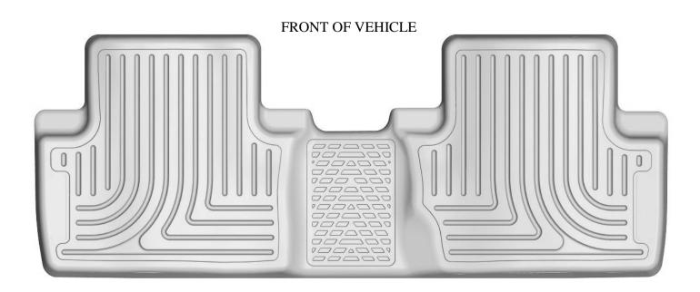
TO EASE INSTALLATION OF YOUR CIVIC 4-DOOR SECOND SEAT LINER, MOVE THE FRONT SEATS TO THEIR MOST FORWARD POSITIONS. WITH THIS DONE, INSTALL THE LINER IN YOUR VEHICLE. ONCE THE LINER IS INSTALLED, REPOSITION THE FRONT SEATS AS DESIRED.
