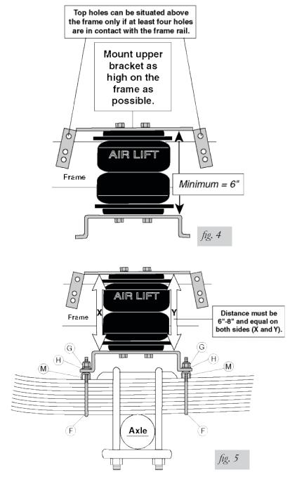
4. Drill the remaining holes. Install the appropriate hardware and torque the nuts to 44 ft.lbs.
