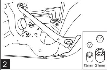
Remove 2 nuts and set assembly into position. Reuse factory nuts and Torque to 41ft-lbs/ 55Nm.
