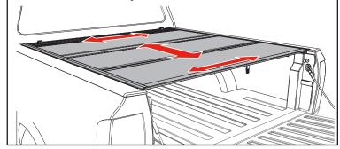
Check if the latches are hitting or not engaging the side rails (A & B) by releasing each latch. If any of the latches need modifications refer to the Slam Latch Adjustment section on the next page on how to make adjustments.
