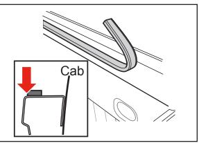
If rubber filler strips (E) were NOT included in your kit, skip to step 3. If you received rubber filler strips (E) with the cover (C), clean the rail the same way as you did in step 1. Peel the backing and adhere the filler strips (E), as illustrated, between the truck plastic bed cap and truck metal rail. Place one 6-8 inches from the bulkhead. Place the rear strip as close to the tailgate as possible. Center the middle strip appropriately.
