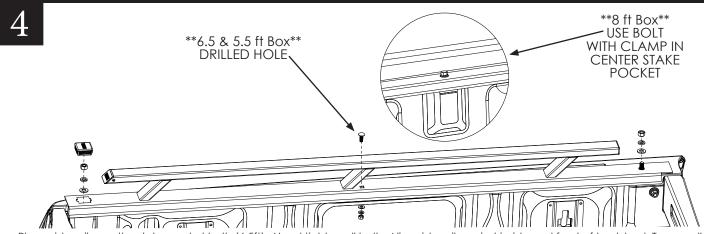
Place side rail over the stake pocket bolts (6.5ft). Hand tighten all bolts. Align side rail against inside and front of truck bed. Torque all bolts. Snap trim cap into rear square hole.
