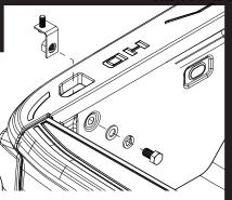
Install rear stake pocket bolt inside pocket. Hand tighten the bolt with lock washer and washer as shown.
