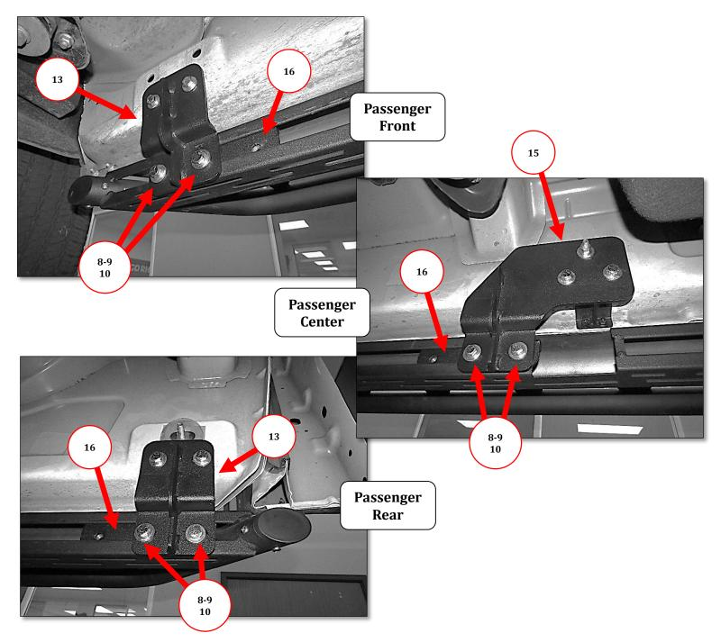
**Step-10** Tighten all bolts securing the Dominator D1 side step to the side step brackets. Repeat the above steps to install the side step brackets and Dominator D1 side step on the driver side of the vehicle. Remember to check and retighten the nuts and bolts every six months.
