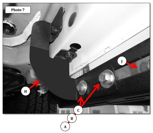
**Step-7** Align the Dominator D1 side step with the vehicle and tighten all bracket and side step nuts and bolts,. Repeat the above steps to install the brackets and Dominator D1 side step on the driver side of the vehicle.
