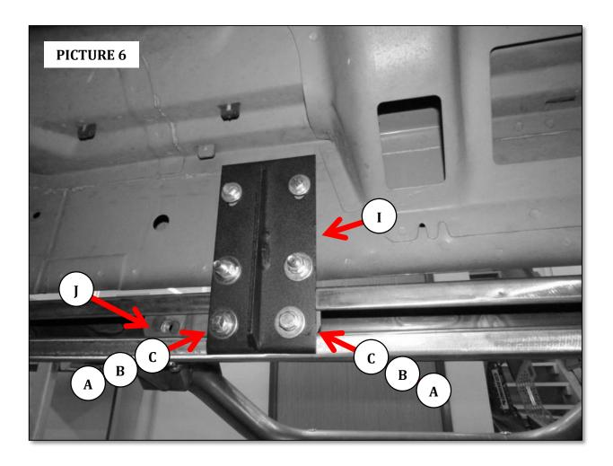
**Step-7** Align the Dominator DSS side step with the vehicle and tighten all bracket and side step nuts and bolts,. Repeat the above steps to install the brackets and Dominator DSS side step on the driver side of the vehicle.
