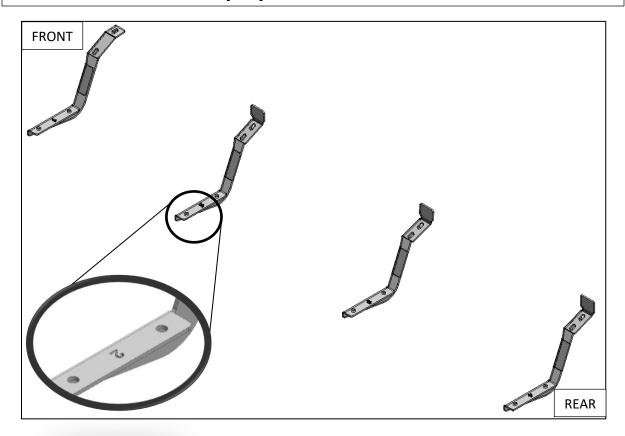
**Step 3:** Set running board along the top of all four brackets and center along the cab.
