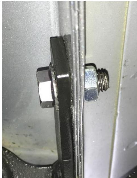
**Step. 7:** After final positioning, completely tighten all (x6) ¼"-20 x ¾" in the pinch weld attachment.
