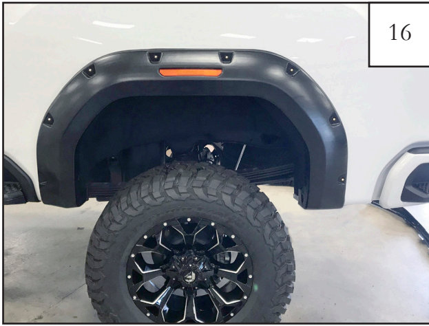
Completed rear flare installation.
