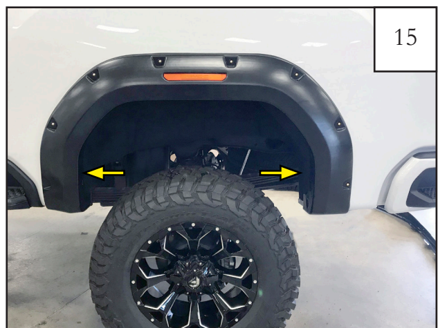
Install (2) panel retainers (RV1-P008).
