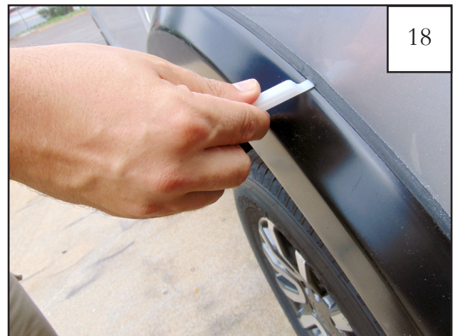
Using flat end of supplied Edge Trim Tool (ET1-0002), seat edge trim against flare by inserting straight end between edge trim and flare at one end. Next, slide around entire edge to the other end.
