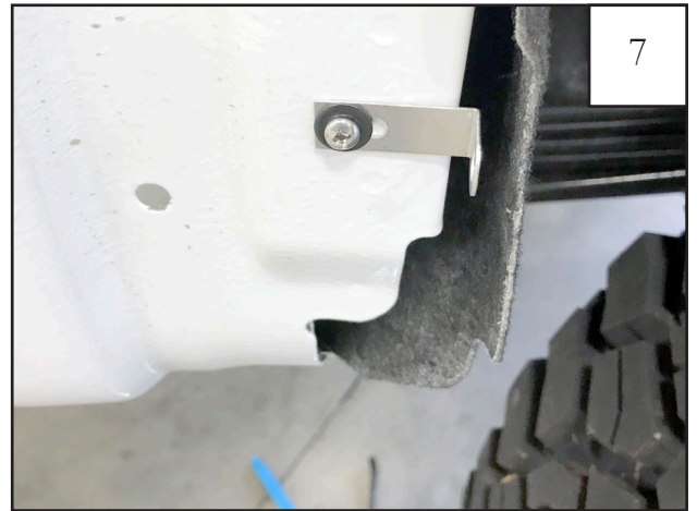
It may be necessary to slightly trim wheel liner so that it does not interfere with mounting hole.
