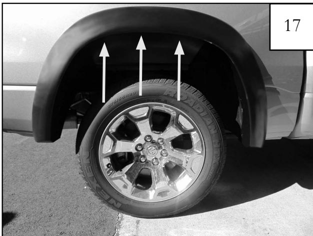
Hold flare in place and reinstall (3) factory screws removed in Step 16. Do not tighten.
