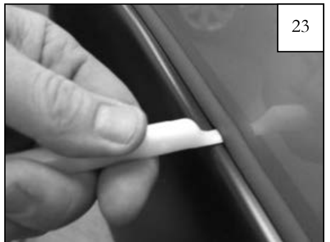
23 Using flat end of supplied Edge Trim Tool (ET1-0002), seat edge trim against flare by inserting straight end between edge trim and flare at one end. Next, slide around entire edge to the other end.
