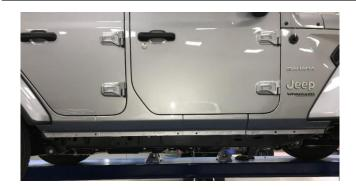
**Step 4:** Carefully raise step assembly into position and align the brackets with the factory mounting points with the horizontal part of the bracket on the outside of the pinch weld.
