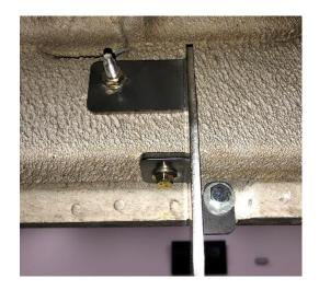
**Step 7:** Set the 31" running board along the top of all 2 brackets and center along the cab.
