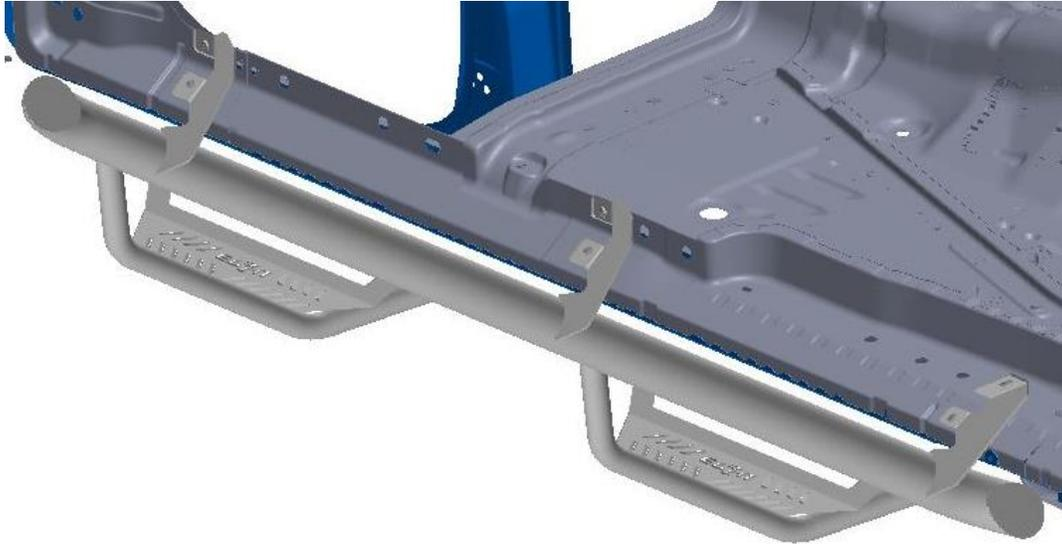
**Step 6.** Next, tighten the three lower bolts first following with the three upper bolts.
