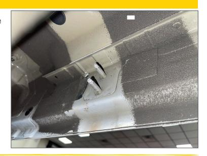
Step 3. Next, place (#1) Driver side step on the studs and secure with supplied (#3,#4) M8 flanged hex nut and M8 flat washer and loosely tighten for now.
