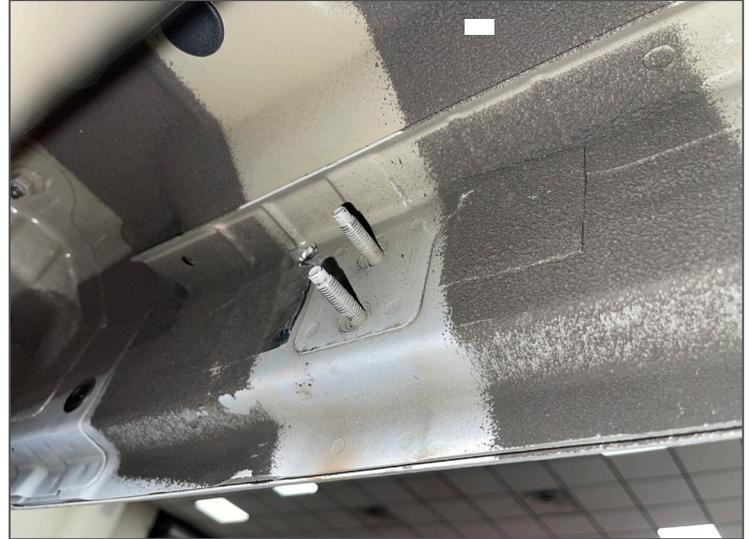
Step 3. Next, place (#1) Driver side on the studs and secure with supplied (#3,#4) M8 flanged hex nut and M8 flat washer and loosely tighten for now.
