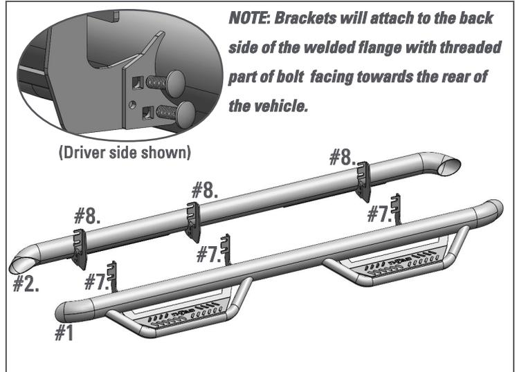
Step 3. Carefully raise Podium step up into position aligning brackets with OE threaded studs and secure with (x6) (#3) M8 hex nut and (x6) (#4) M8 flat washer and hand tighten for now.
