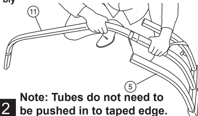
**Note: Tubes do not need to be pushed in to taped edge.**
