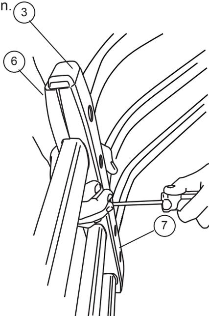
**8** **NOTE:** Do not over tighten as this may strip out. Fastener will reach a noticeable stopping point.
