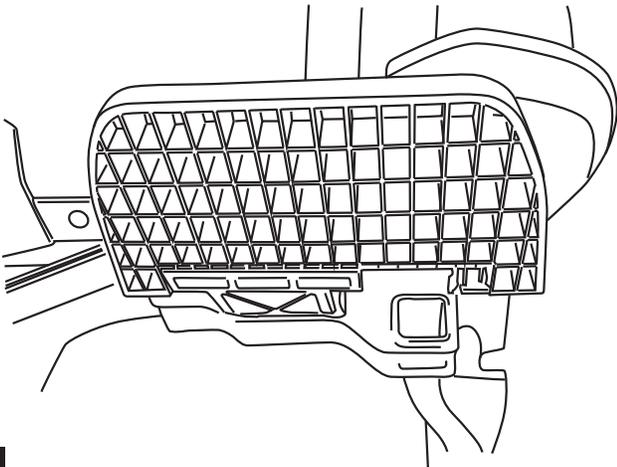
Torque 3 PT screws to 5 ft-lbs / 6Nm
