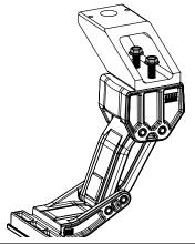
Using a 13mm Socket assemble Frame mount onto Lateral mount. Do not tighten bolts yet.
