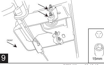
For 2011 - up Short bed models: Remove the two rearmost u clips off the bracket and change orientation of the bolt so that the bolt head is on the outside of the bracket. Torque bolts to 16 ft-lbs.
