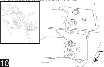
For 2011 - up Short bed models : Attach bracket to threaded hole in frame mount. Rotate bracket up to position and use provided M12 Hardware. Tighten M8 bolt to 16 ft-lbs and M12 bolt to 35 ft-lbs.
