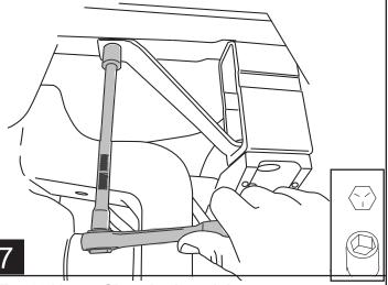
For 2011 - up Short bed models: Using a 15mm socket remove four bolts holding factory bracket in place. The two rear most U clips will need to be removed in step 10. For all other models skip to step 10.
