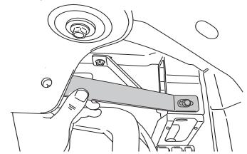
12 NOTE:If a hole is not provided on a factory body mount, a hole must be drilled using a 1/2" drill bit.
