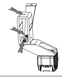
Using a 15mm socket with extension, align bolt with threaded plate. Do not tighten.
