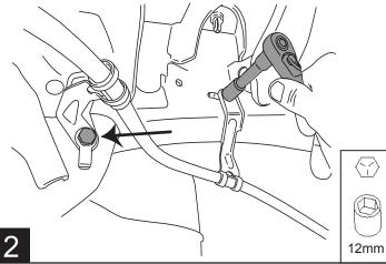
Using a 14mm wrench remove body mount bolt.
