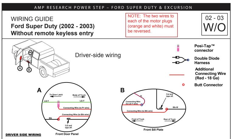
1. Remove door panel, access a bundle of wires below and to the left of speaker (Area-A). Open bundle and locate 18Ga. door-ajar wire ( light areen with yellow stripe).
