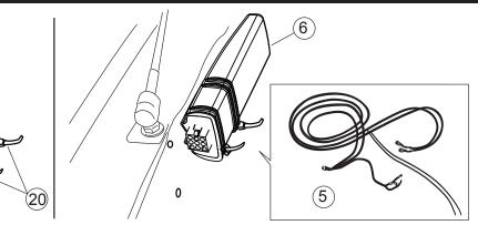
Loop two large tie wraps through fastener cutouts in sheet metal as shown. Position controller as shown above and cinch down tie wraps to secure controller in place. Connect harness to controller. Make sure that locking tabs on controller/harness connector are fully engaged.
