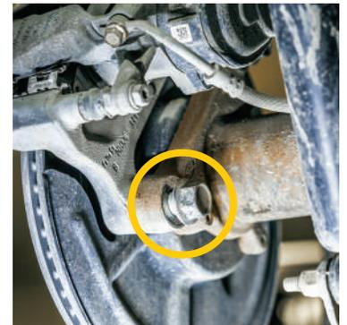
3. Position the guard in front of the train axle & slide the top open tab hole of the guard into the top caliper bolt. Swing the bottom open tab hole of the guard into the bottom caliper bolt. (\*Please note: it's important to install the top mount first).
