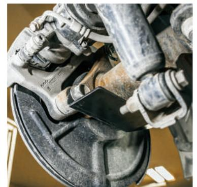
4. Ensure to make the two open tab holes sit against the caliper bolts before re-tightening the bolts to the factory specs.
