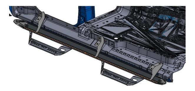
**Step 5:** Next, tighten the three lower bolts first following with the three upper bolts.
