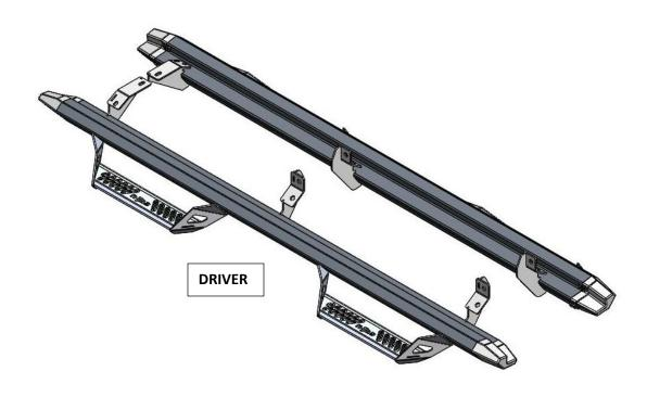
**STEP 2:** Remove any factory running boards or hardware and discard. **STEP 3:** Clean/tap the three factory threaded mounting locations.
