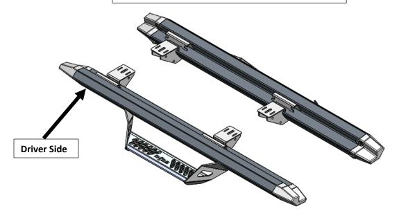
**Step. 3** Starting with the passenger side step rail, install the supplied (x6) 5/16" snap nuts into the two notches in each mounting bracket.
