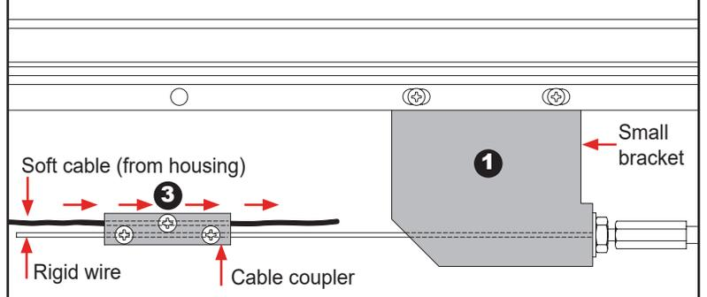
**OPERATING THE OVERRIDE - Use only when the cover is not operating remotely.**
