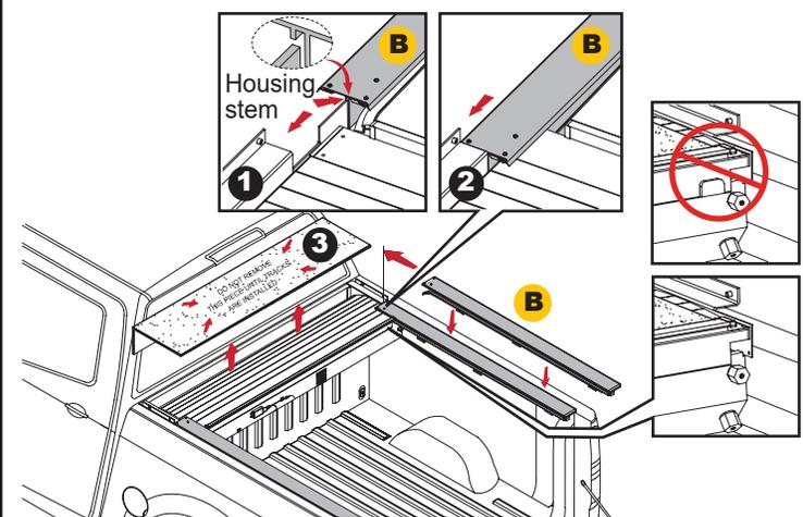
**9** (1) Loosely attach the CM track bracket (E) to the pre-installed track clamp with 1/4" flat washer (N) and 1/4" socket cap screw (M). (2) Loosely attach CM bed clamps (F) to the pre-installed track clamps using 5/16" socket cap screw (K) and 5/16" lock washer (L) on driver and passenger side.
