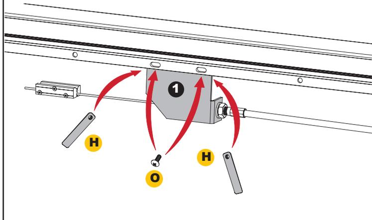
Attach large bracket (2) through the slotted holes using two cargo nuts (H) and two 10-24 screws (O) towards the back of the track.
