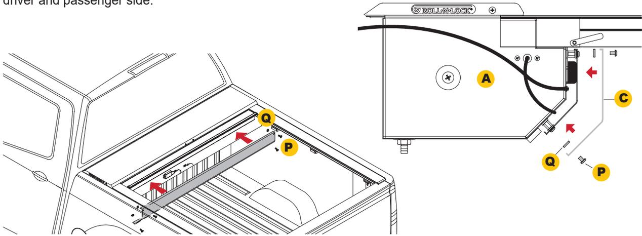
**19** Drill 1/2" hole (1) through bulkhead as shown on driver and passenger side. **DO NOT** drill through the truck cab. Insert one end of the drain tube (D) through the drilled 1/2" hole and feed toward the ground and insert the other end onto the housing fitting. Make sure the drain tubes (D) are **NOT** aligned with or through the cab vents (2) on driver and passenger side. **Note:** Rust protection should be used on the holes drilled.
