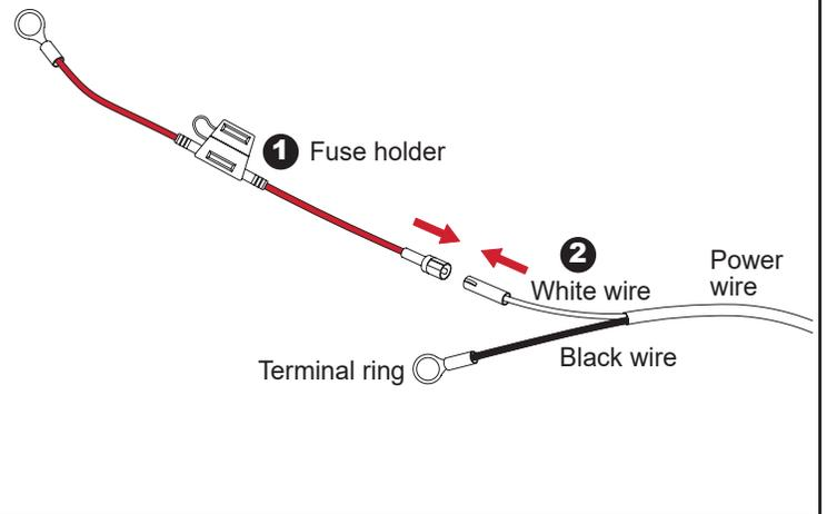
**4** Connect the red fuse holder ring to positive terminal (1) and the black wire/terminal ring to negative terminal (2) of battery.
