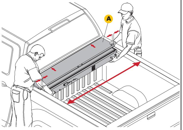
**6** Remove lid from housing (A) by pushing toward cab (1) and up (2) on driver and passenger side.
