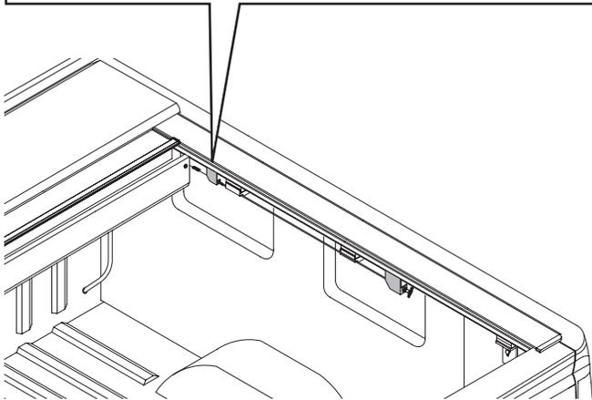
Loosen top screw (3), pull the soft cable from the housing taught through the cable coupler and tighten screw.
