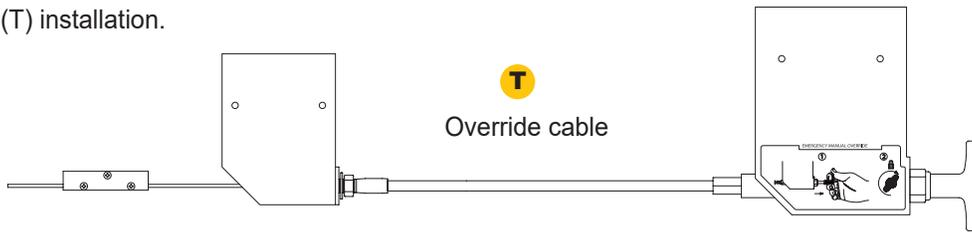
Attach small bracket (1) through the slotted holes using two cargo nuts (H) and two 10-24 screws (O) towards the front of the track.
