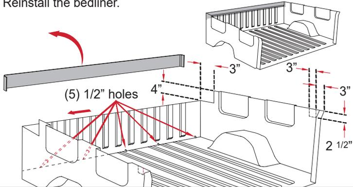
**1B** Drill 1/2" hole through plug (only) on back of truck bed and feed end of power wire between truck bed and cab, letting the wire continue to the ground. Leave 3' of power wire in the truck bed.
