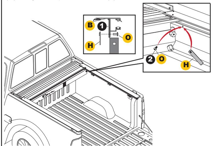
**11** Close tailgate, shift the housing (A) back so the end of the tracks (B) are up against the tailgate on driver and passenger side.
