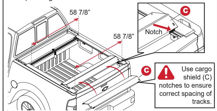
**11A** WITH MULTI-FLEX/MULTIPRO TAILGATE ONLY - With track (B) correctly back against tailgate height tighten #10-24 screw. Adjust track to correct height and tighten nut (1) on driver side only.
