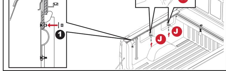
**7B** Loosely attach the track bracket (F) to the pre-installed track clamps with 1/4" flat washer (I), 1/4" lock washer (N) and 1/4" socket cap screw (M). Loosely attach bed clamps (J) to the pre-installed track clamps using 5/16" socket cap screw (K) and 5/16" lock washer (L) on driver and passenger side.
