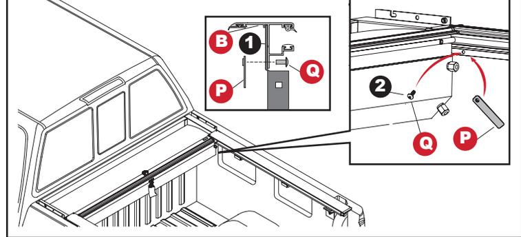
**9** Close tailgate, shift the housing (A) back so the end of the tracks (B) are up against the tailgate on driver and passenger side.
