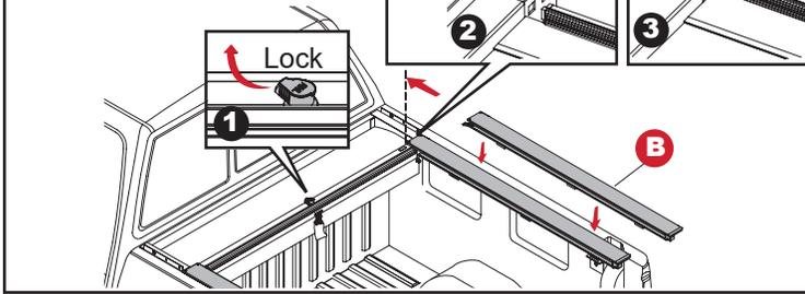
**7A** WITH MULTI-FLEX/MULTIPRO TAILGATE ONLY - Align track clamp (X) over screw on Multi-Flex/MultiPro step handle bracket, replace nut and washer loosely (1) on driver side only. Loosely attach the bed clamps (J) to the track clamps on driver side only.
