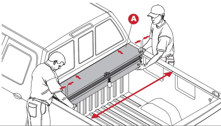
**3** Remove lid from housing (A) by pushing toward cab (1) and up (2) on driver and passenger side.
