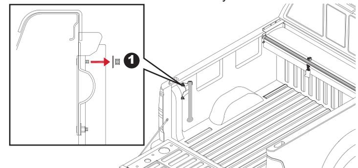
**6B** (1) Turn lock to 10 o'clock. (**Do not remove plastic wing nut**). (2) Align tracks (B) onto housing stem. (3) Make sure the edge of the tracks butt up against housing on driver and passenger side.
