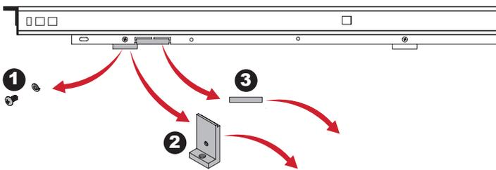
**4B** WITH MULTI-FLEX/MULTIPRO TAILGATE ONLY - Align track clamp (X) onto the back of the track at the slotted hole. Using the same screw and washer that was removed, loosely attach bracket to track on driver side only.
