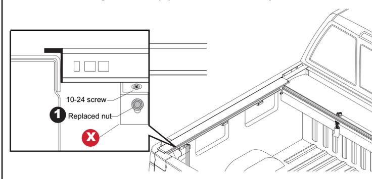
**11B** Once tracks (B) are correctly spaced and adjusted to the correct height, tighten back clamp (F) with fastener (M) using a 3/16" Allen wrench (1) and fastener (H) using a 7/16" wrench (2) on driver and passenger side.
