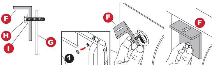
**6A** WITH MULTI-FLEX/MULTIPRO TAILGATE ONLY - Remove nut and washer (1) from the top of the step handle bracket on driver side only.
