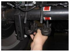
Remove u-bolt nuts and lower plate.
