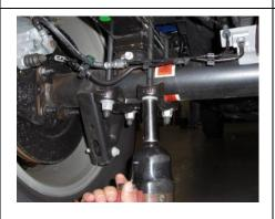
Loosen and remove factory u-bolt hardware.
