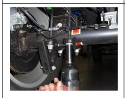
Loosen and remove factory u-bolt hardware.
