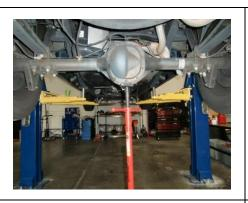
Raise vehicle securely by frame and support axle with jack..
