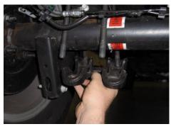
Remove u-bolt nuts and lower plate.
