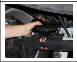
Install lift block with centering pin toward axle.
