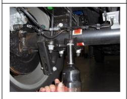
Loosen and remove factory u-bolt hardware.
