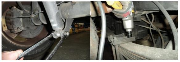
Remove the lower shock mount hardware.
