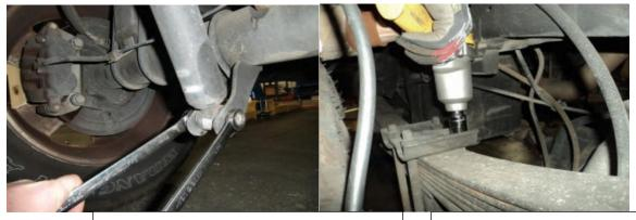
Remove the lower shock mount hardware.
