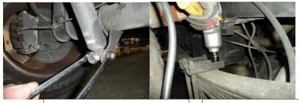
Remove the lower shock mount hardware.
